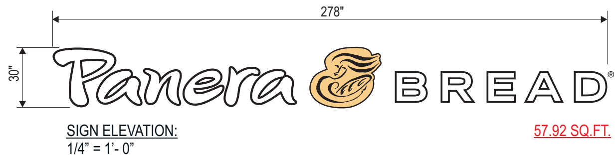
INDIVIDUAL ILLUMINATED GRAPHICS - LETTERS AND LOGO: FACE-LIT AND HALO LIT CHANNEL LETTER CONSTRUCTION:
