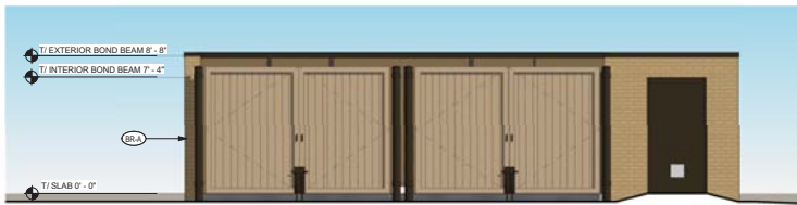
REFUSE ENCLOSURE ELEVATION - FRONT 1/4" = 1'-0"
