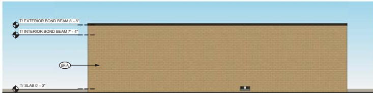
REFUSE ENCLOSURE ELEVATION - REAR 1/4" = 1'-0"
