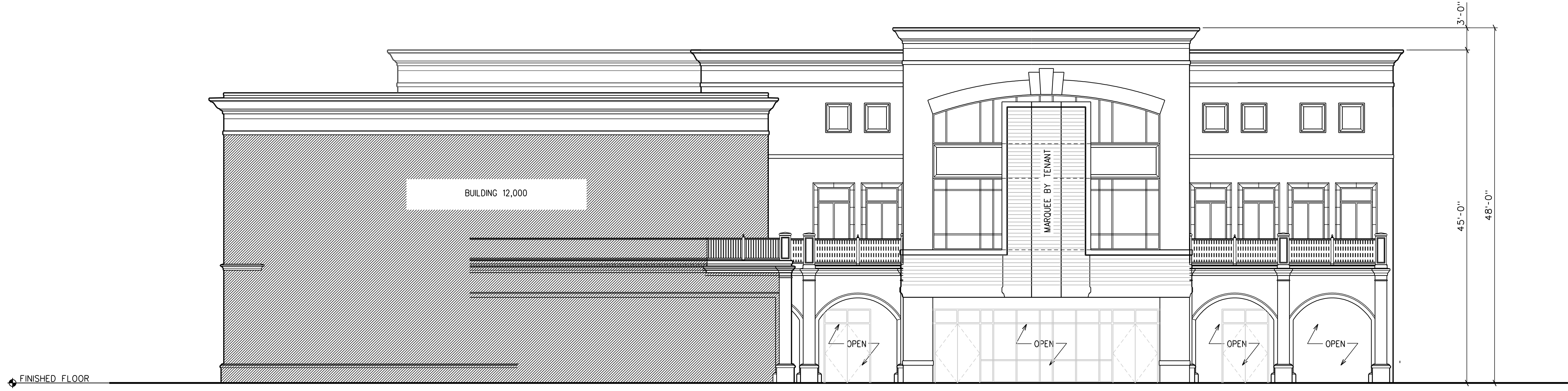
1 WEST ELEVATION (FACING WATER FEATURE): BUILDING 14,000 SCALE : 1/8" = 1'-0"
